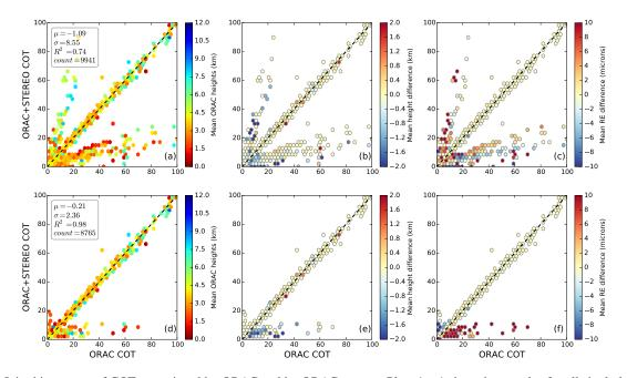
**Figure 10.** Joint histograms of COT as retrieved by ORAC and by ORAC+stereo. Plots (**a**–**c**) show the samples for all single-layer clouds over water (number of layers determined by CALIOP and open water determined by AMSR-E). Plots (**d**–**f**) show the subset of the sample where the ORAC and ORAC+stereo phases are in agreement.
