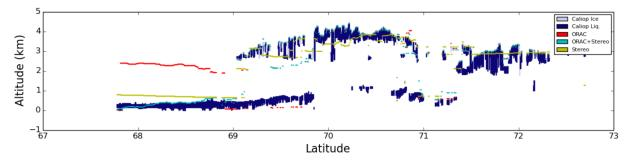
Figure 5. This profile plot show the 1 km CALIOP cloud profile for orbit with the time stamp 2008-07-05T13-02-15ZD. Over plot are the collocated CTH data from ORAC, ORAC+stereo, and census stereo. The key in the plot indicates the relationship between colour and feature type.
