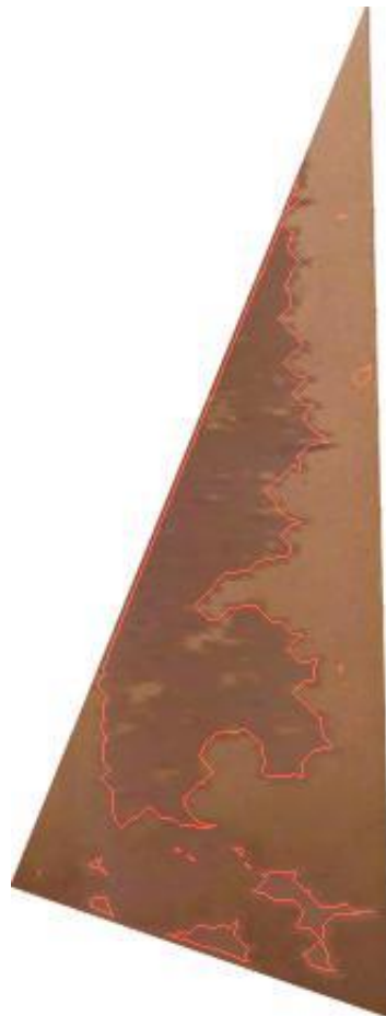
Figure 10. The upper-right triangle of new image of test 2: the stain is well detected and isolated.
