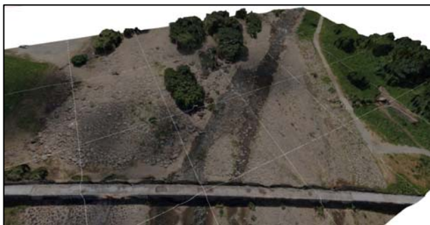
Figure 18. DSM generated with images from UAV
