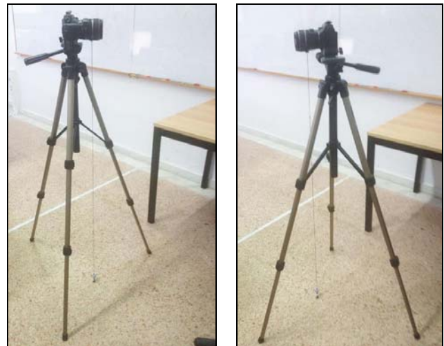
Figure 10. Image acquisition; keeping constant the same ground point at each shoot.
