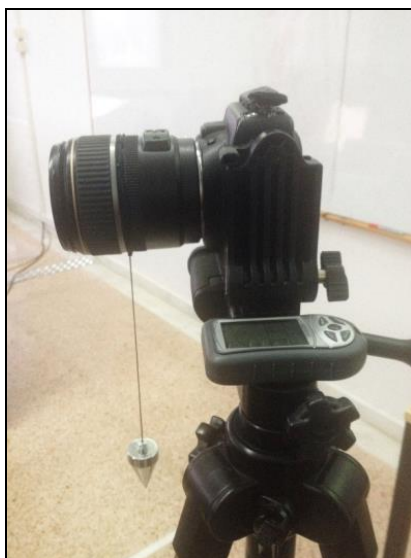
Figure 9. Camera position over the tripod, the plump line and the electronic compass.
