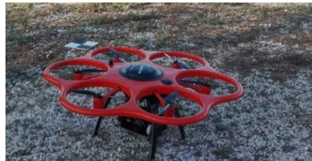
Figure 6. The hexacopter Aibot X6 V2 by Aibotix.
