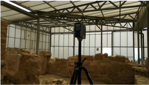
Figure 10. Laser scanning survey.
