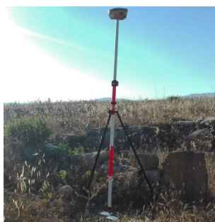
Figure 5. NRTK survey with Topcon HiperV GNSS receiver.
