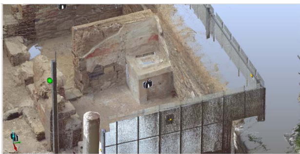
Figure 11. A detail of scan and targets positions.
