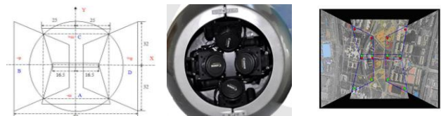
Figure 3. The structure of the designed four-combined wide-angle camera(Unit: mm, view angle: 100^\circ \times 130^\circ )
