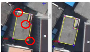
c. The polygon and right-angle roof building measurement
