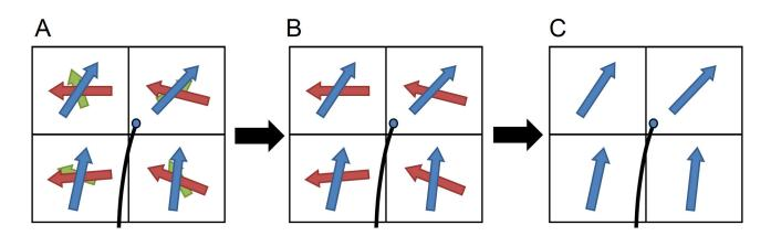
**Figure 2.** The filtering-selection process used in the generalized deterministic fiber tracking algorithm. (A) Each voxel may resolve multiple fiber orientations. (B) The noisy fibers are filtered using a pre-defined QA threshold. (C) The fiber orientations forming the least turning with respect to current propagation direction are selected. doi: 10.1371/journal.pone.0080713.g002
