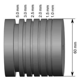
**Figure 4. The design of a phantom spindle.** The phantom has six different sized grooves wound with polyester fibers to examine the spatial resolution of a fiber tracking algorithm. (Bach Micheal et al., "DWI-Phantom–Resolution Phantom", http://www.nitrc.org/ projects/diffusion-data , use with permission). doi: 10.1371/journal.pone.0080713.g004
