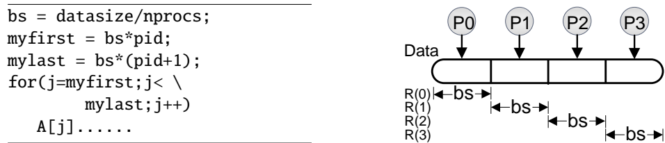
Figure 52: Example TI structure and the corresponding block pattern ( nprocs = 4 )
