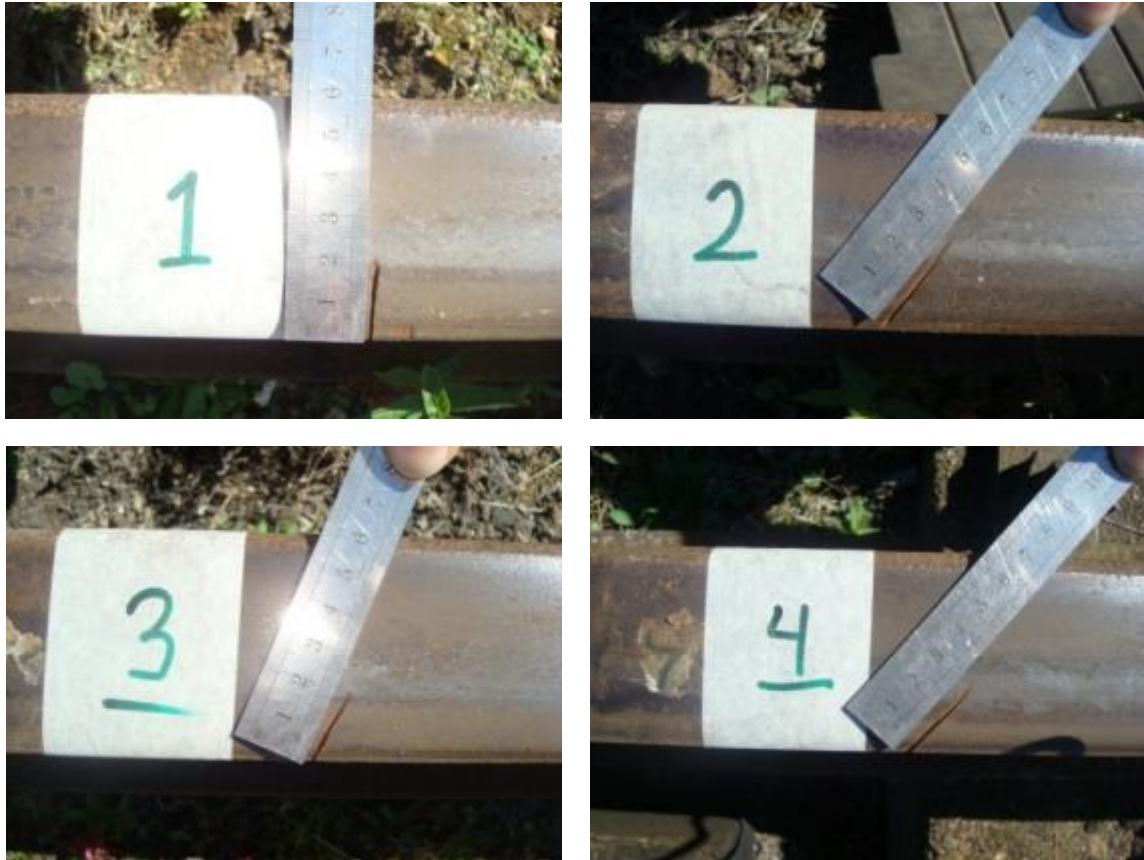
Figure 5.6 The artificial defects of varying geometries on the rail track. The numbers represent the order in which the defects appear relative to the fixed datum.
