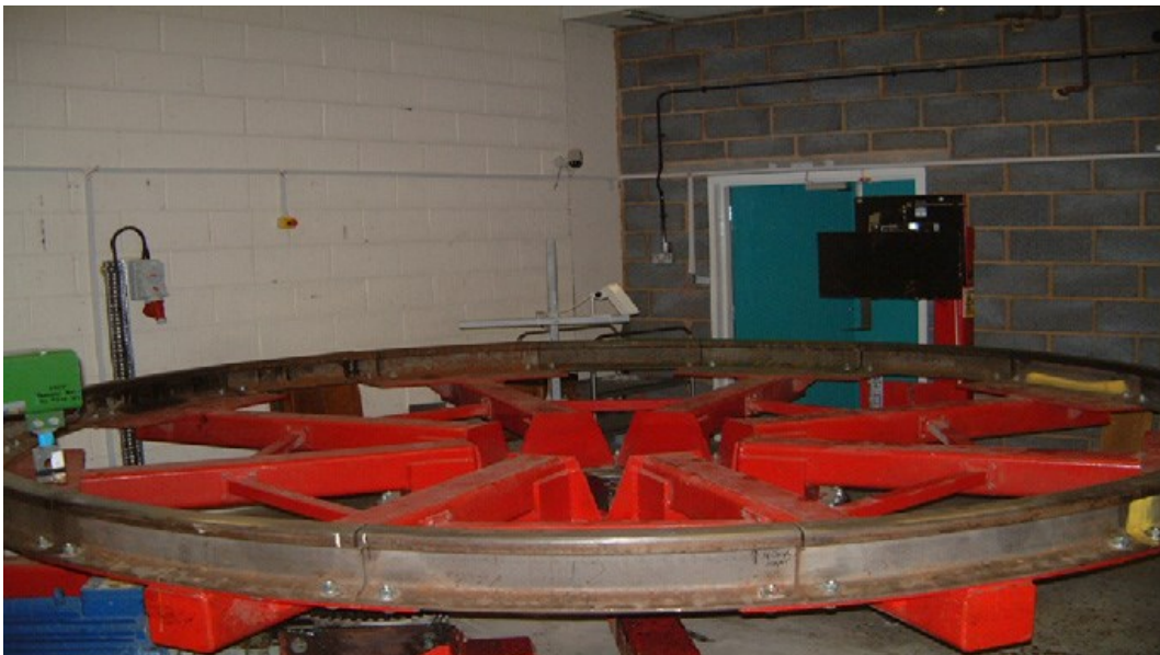
Figure 5.10 Illustration of the rotary rail rig at the University of Birmingham used for high speed ACFM measurements [56].
