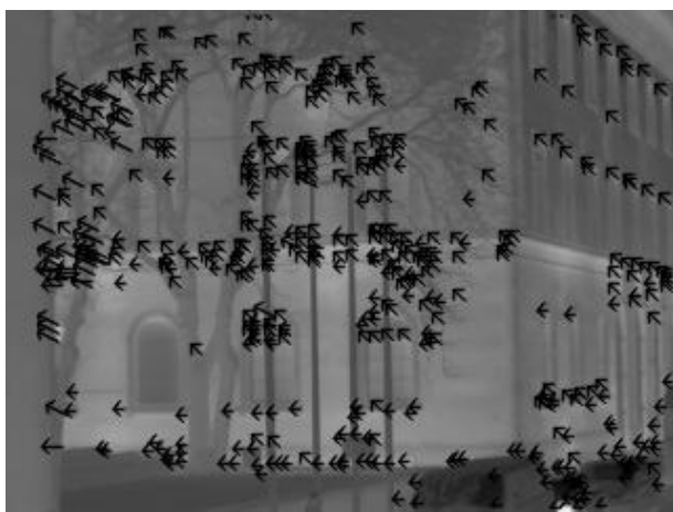
Figure 2. IR image with selected SIFT features, that have correspondences in the following image. Arrows show the moving direction of the points and numer of pixels they move.
