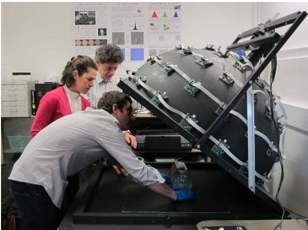
Figure 6. Placing the handbag on the baseplate of the UCL dome. For photography the hinged upper part was lowered onto the frame, so that the object was completely enclosed. Photograph by Jananne Al-Ani.
