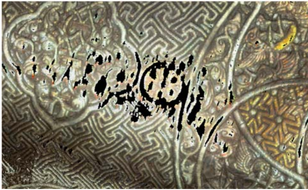
Figure 2. 'Holes' in the point cloud produced by the Arius 3D scanner in curved regions of high specularity.
