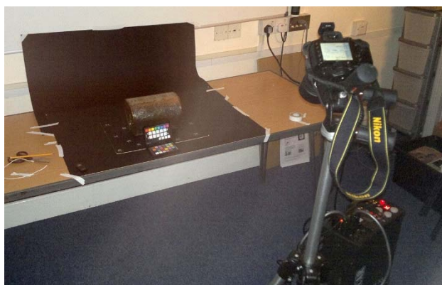
Figure 3. Setup for photography of the handbag, showing cove, colour chart, camera on tripod and flash controller.
