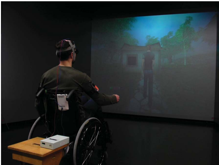
Fig. 1. The experimental set-up. An inertial sensor (MTx miniature inertial measurement unit, Xsens Technologies BV, Enschede, the Netherlands) was attached to the subject's right upper arm. A dummy sensor was attached to the left upper arm to avoid focusing on one arm. The virtual reality system was controlled by D-flow software (CAREN, Motek Medical BV, Amsterdam, the Netherlands), and the virtual scene was projected in 3D (2 projectors, CP-WX8255A, 1920 × 1080 High Definition, Hitachi, Tokyo, Japan) on a large silver-coated projection screen (projection surface 3.05 m × 2.06 m). The inertial sensor was connected to the virtual reality system via a wireless Bluetooth connection. The rotation data for the sagittal plane, acquired with the inertial sensor, was used to animate the progress bar in the lower left corner. In addition, during avatar trials the same signal was used to go through a pre-programmed walk-cycle animation of the avatar.
