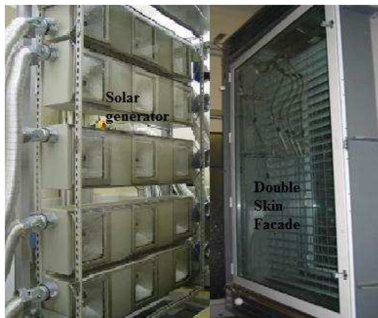
Figure 8-5: Test chamber showing solar generator and DSF , Mei et al. [290]
