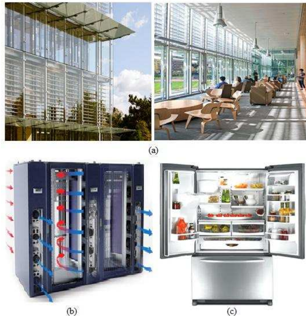
Figure 1-2: Examples of natural convection systems: (a) Indoor environment [23], (b) Electronic devices [24], (c) refrigerator with food arrangement [25].
