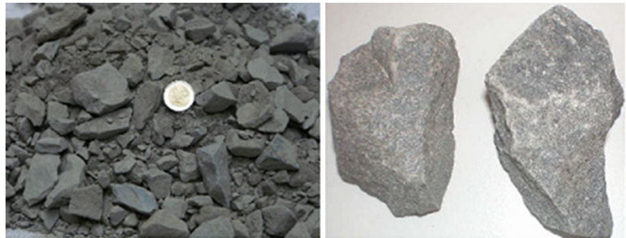
Fig. 1 South African crushed stone (G1) material details
