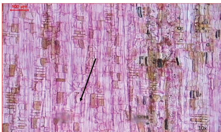
FIGURE 1. Longitudinal section of compreg Mahang taken near the surface of sample. The resin solid content (arrow) was deposited in the cell lumens
