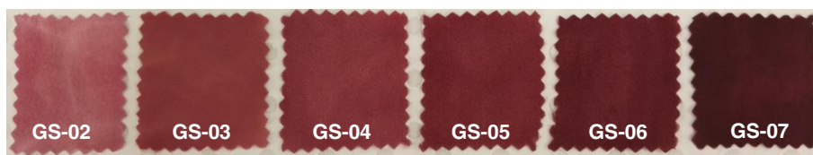
Fig. 1 Optical images of the silk fabrics treated with different concentrations of \text{HAuCl}_4 solutions
