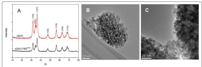
**Fig. 1** Crystal phase composition, size, and morphology characterization for nZnO and nZnO – FBS<sup>dried</sup> NPs. **a** XRD spectra and TEM images for **b** nZnO and **c** nZnO – FBS<sup>dried</sup>
