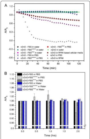
**Fig. 4** Sedimentation profile evaluation for NP stock dispersions. Sedimentation profiles of 25 mM ZnO stock dispersions (pH = 7.3) for a 2-h time period. **a** nZnO, nZnO – FBS<sup>dried</sup>, nZnO – FBS<sup>washed</sup>, and nZnO – FBS stock dispersions in various biologically relevant solutions. **b** Sedimentation histograms for 0, 0.5, 1.0, 1.5, and 2.0-h time points for nZnO – FBS<sup>dried</sup>, nZnO – FBS<sup>washed</sup>, and nZnO – FBS stock dispersions in PBS and nanopure water
