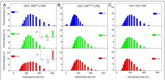
**Fig. 6** Hydrodynamic size distribution profiles at 0, 12, and 24 h. Histograms represent 25 mM stock dispersions prepared in PBS for **a** nZnO – FBS<sup>dried</sup>, **b** nZnO – FBS<sup>washed</sup>, and **c** nZnO – FBS
