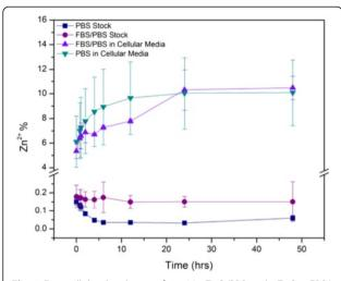
**Fig. 9** Extracellular dissolution of 6 mM nZnO/PBS and nZnO – FBS/PBS stock dispersions and 0.6 mM of those respective nZnO stock dispersions in RPMI-based cellular media.  $Zn^{2+}$  concentration is expressed as %  $Zn^{2+}$  (total dissolved  $Zn^{2+}$  measured by ICP-MS/total  $Zn^{2+}$  in sample) to normalize for concentration
