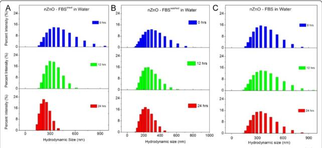
Fig. 7 Hydrodynamic size distribution profiles at 0, 12, and 24 h. Histograms represent 25 mM stock dispersions prepared in water for **a** nZnO – FBS<sup>dried</sup>, **b** nZnO – FBS<sup>washed</sup>, and **c** nZnO – FBS
