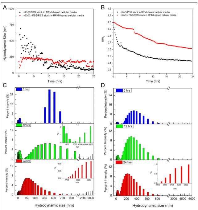
**Fig. 8** Dispersion stability analysis for nZnO/PBS and nZnO – FBS/PBS stock solutions introduced to RPMI-based cellular media at a concentration of 0.6 mM. **a** Average hydrodynamic size profiles for a 24-h time period. **b** Sedimentation profiles for a 24-h time period. Hydrodynamic size distribution profiles at 0, 12, and 24 h for **c** nZnO/PBS stock dispersion in RPMI-based cellular media and **d** nZnO – FBS<sup>′</sup>PBS stock dispersion in RPMI-based cellular media
