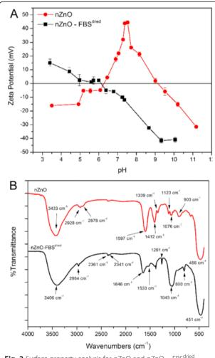
**Fig. 2** Surface property analysis for nZnO and nZnO – FBS<sup>dried</sup>. **a** Zeta potentials measured as a function of pH and **b** FTIR spectra with the wavenumbers of the main peaks marked
