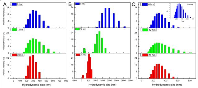
Fig. 5 Hydrodynamic size distribution profiles at 0, 12, and 24 h. Histograms represent 25 mM stock dispersions prepared in **a** nanopure water, **b** PBS, and **c** RPMI-based cellular media
