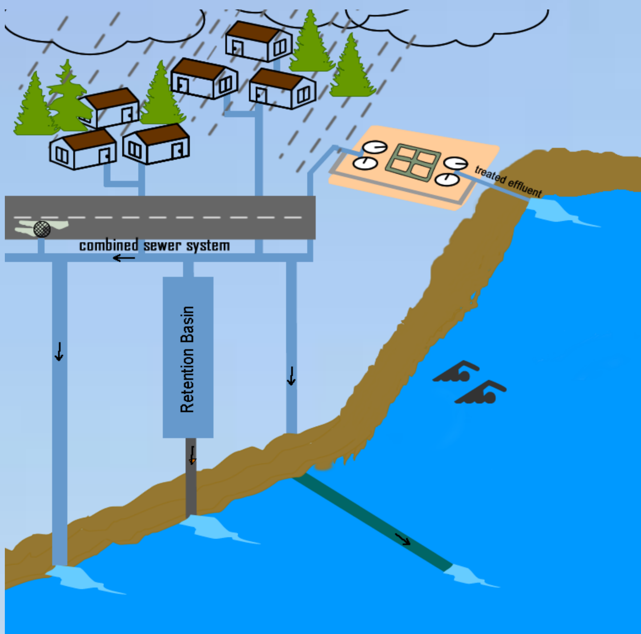
Figure 1: Schematic representation of combined sewer overflows
