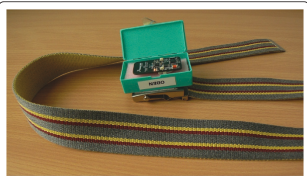
Figure 1 Triaxial accelerometer sensor ( Freescale RD3152MMA7260Q ), sensor casing and belt. No skin contact is necessary for the sensor function
