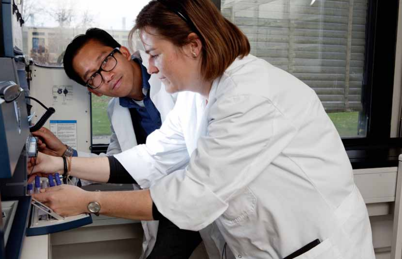
Postdoc Marcel T. Ale is watching how lab technician Annette Eva Jensen loads samples for biomass monosaccharide composition analysis by HPAEC-PAD. This analysis is an important base for designing enzyme reactions on biomass.
