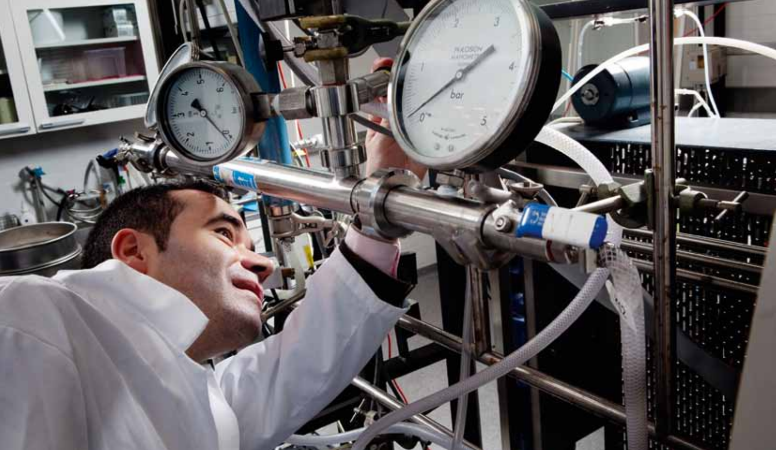
Associate Professor Manuel Pinelo working on ultrafiltration hollow fiber membrane used for continuous separation of bioactive compounds.
