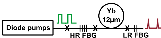
Fig. 1. Yb-doped fiber laser pumped by the diode pumps that are spliced to a high reflector fiber Bragg grating (HR FBG). A varying length of Yb-doped fiber is spliced to the HR and the low reflector grating (LR FBG). By modulating the pumps the laser produces stable pulses.
