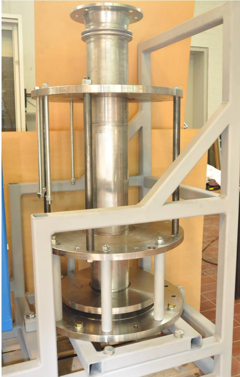
Figure 4.5: The cryostat. - The cryostat, 1.15m high, is lowered into the armature bore from the top. The bottom torque transfer element and bottom of the cryostat have corresponding pins and slots which are making sure that the cryostat is placed in the axis of rotation.
