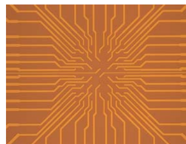
Figure 1. Optical micrograph of a micro-electrode array (MEA) fabricated on thermally oxidized silicon wafer (2.5 \mu\text{m} of oxide), with leads made of sputtered TiW (120 nm) and silicon nitride top coating (100 nm).
