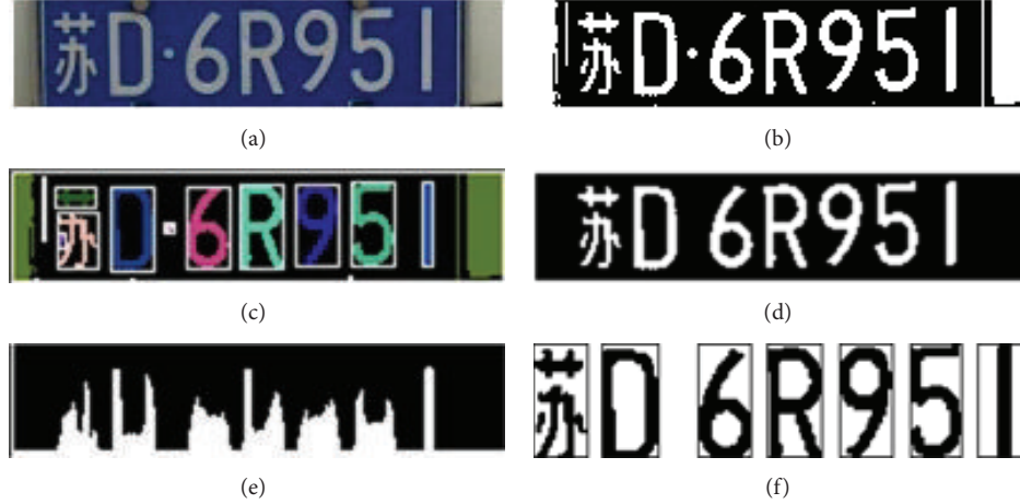
FIGURE 10: The effective images in the process of character segmentation (zoom shown). (a) Original image. (b) Binary image. (c) Connected component labeling. (d) The result of eliminating noise. (e) The projection histogram. (f) The resulting image of segmentation.
