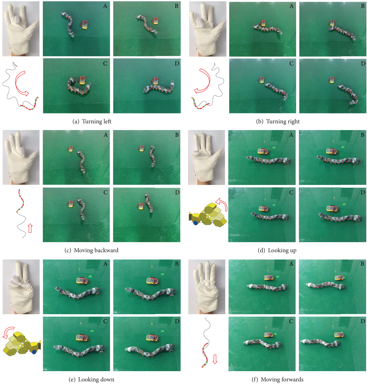
FIGURE 12: Snake-like robot gesture control experiments.
