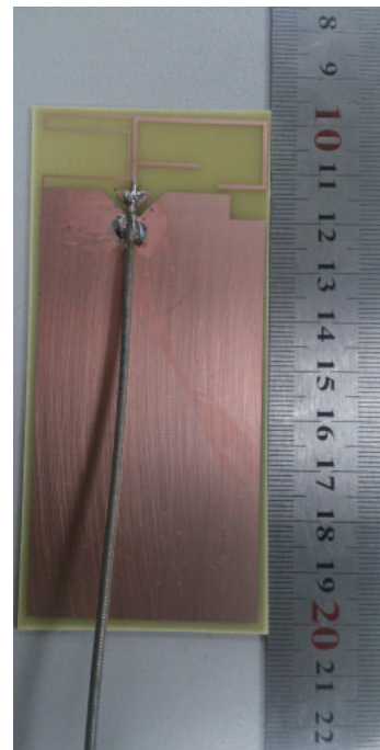
FIGURE 9: Fabricated prototype of the proposed antenna.
