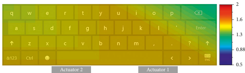
FIGURE 12: Equalized acceleration distributed on the touchscreen by the tactile force adjustment function that computes globally equalized tactile forces concerning the distance between actuators and key locations.
