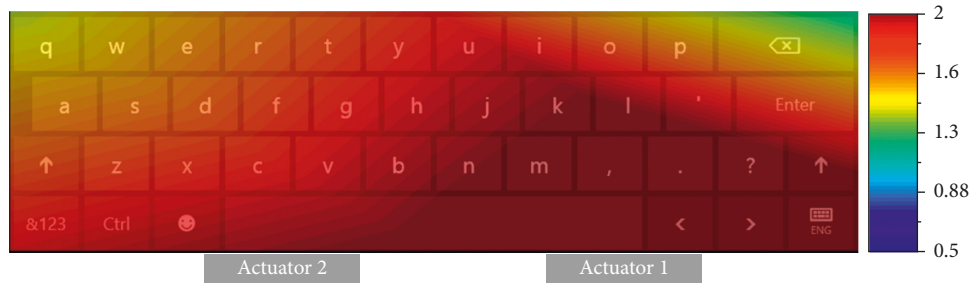
FIGURE 11: Acceleration distributed on the touchscreen of the tablet (Mu Pad): the measured values were superimposed onto the soft keyboard image to visualize the tactile strength generated from two piezoelectric actuators attached on the bezel. Note that red means stronger tactile feedback.
