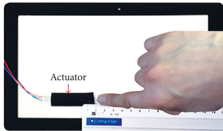
FIGURE 8: Experimental setup of a perception study on key click tactile feedback.
