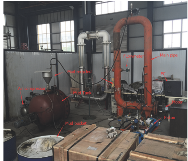
FIGURE 11: Experimental platform of the deep-water drilling gas kick.
