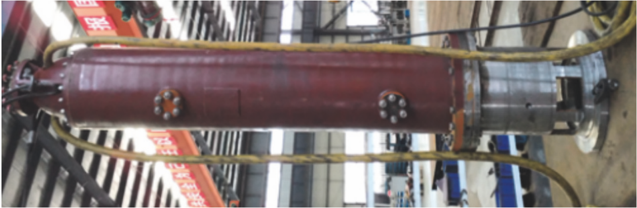
(b) External view of the model rescue pump
