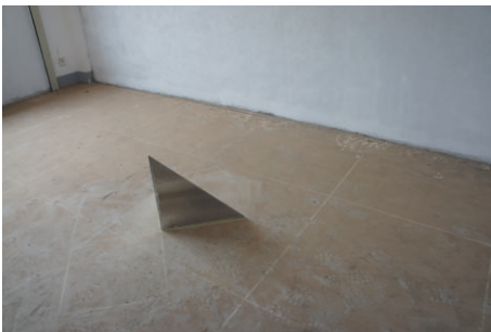
FIGURE 20: In the static target experiment, a trihedral is used as the target and placed 2 m behind the wall.
