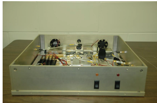
FIGURE 5: Fully packaged S-Band radar system (minus antennas).
