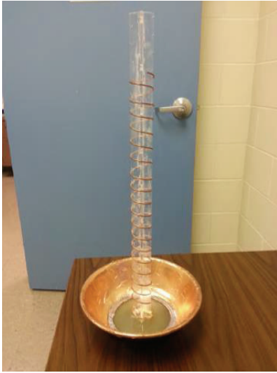
FIGURE 6: View of the helical antenna showing the construction details.
