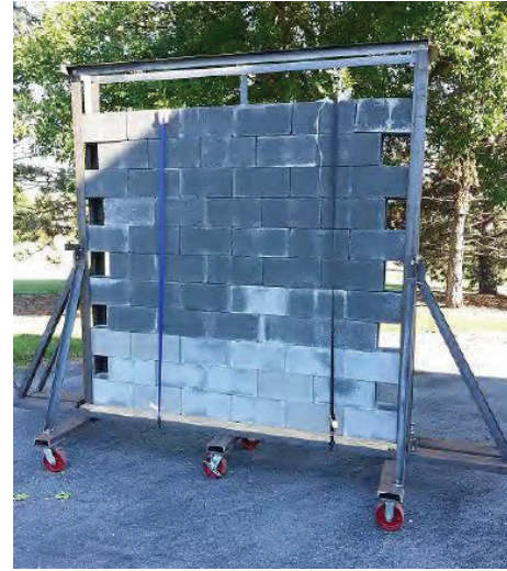
FIGURE 7: 20.32 cm (8 in) thick cinder block wall in the wall support frame.
