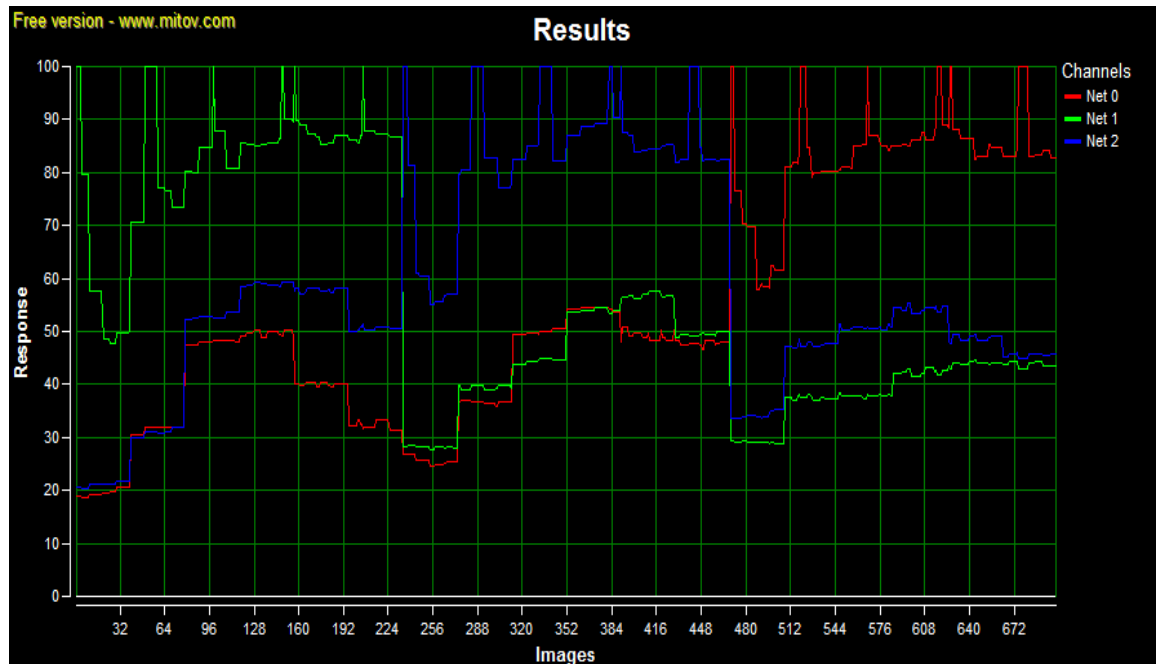
Figure 7.16 - Results of zoom test on 3 subjects, 6 images per subject trained on, and 702 images tested on
