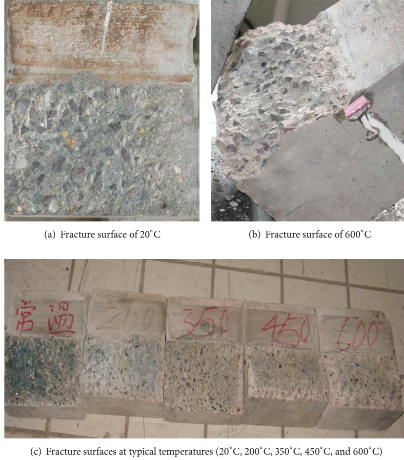
FIGURE 5: Fracture surfaces of postfire specimens.
