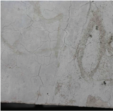
FIGURE 4: Microcracks on specimen surface (600°C).
