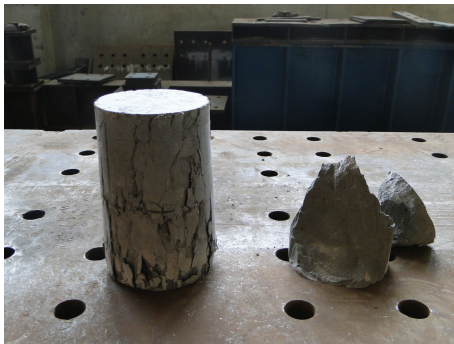
FIGURE 3: Failure of specimens under uniaxial compression.
