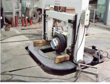
FIGURE 2: Analytical tire contact system.
