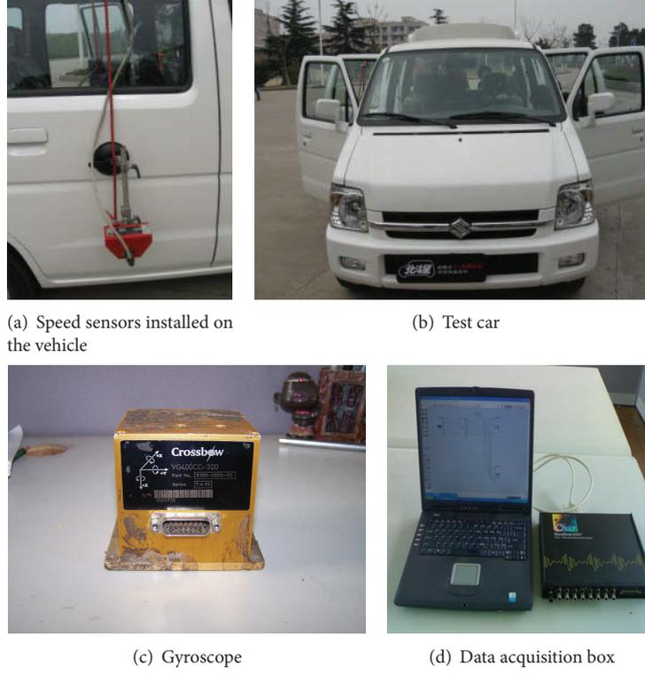
FIGURE 15: Main parts of the test and control systems.
