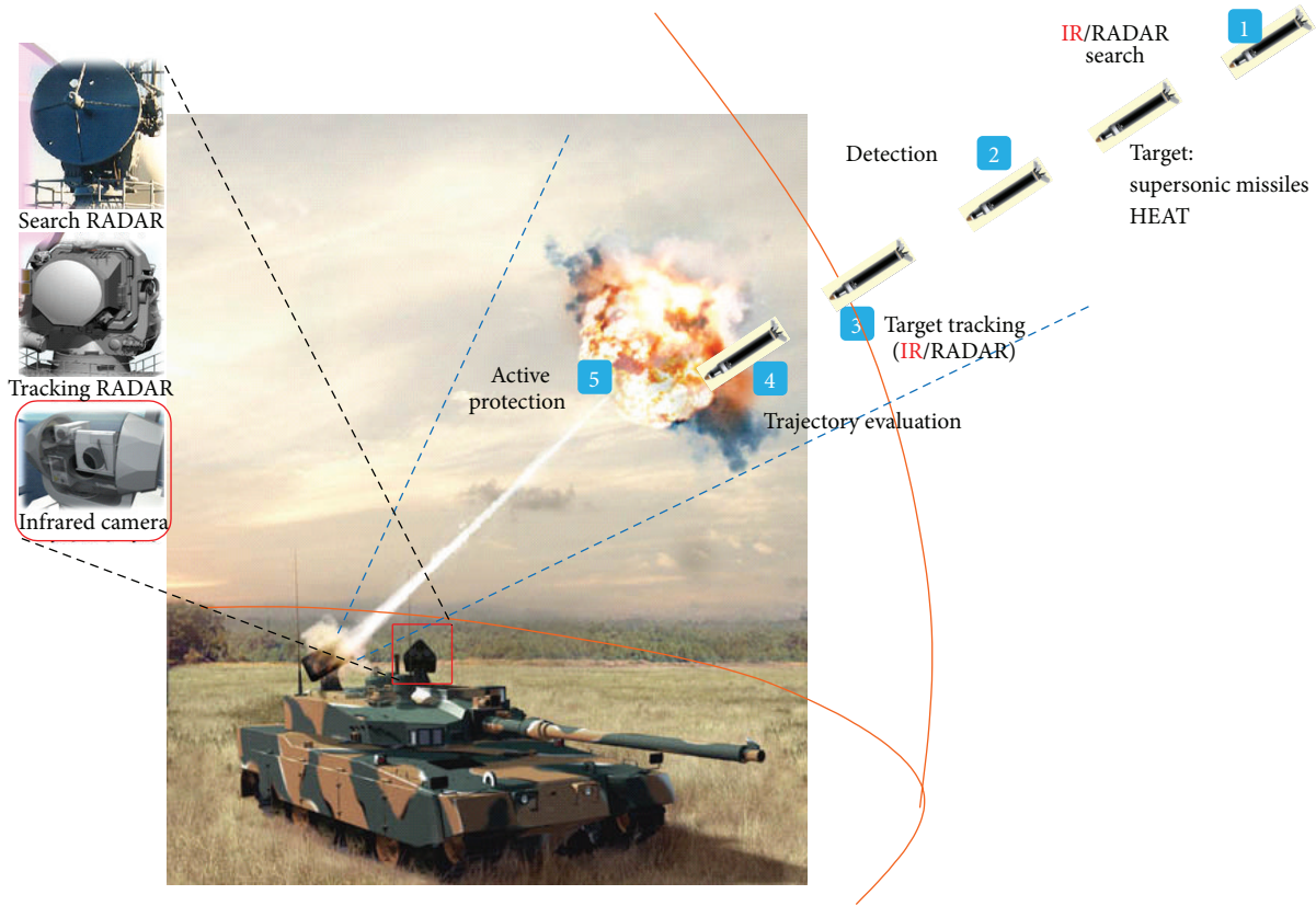
FIGURE 1: IR-based target detection and tracking in active protection system (APS).
