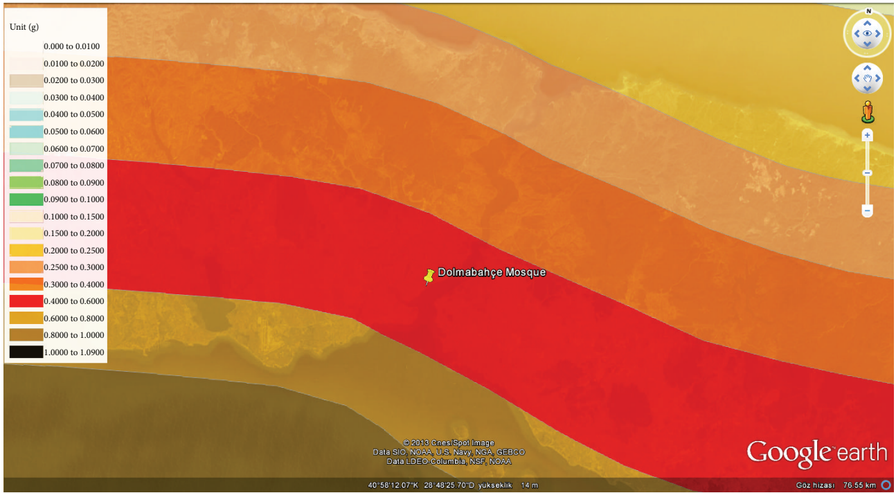
FIGURE 7: Maximum peak ground acceleration map for 475 years return period (10% exceedance in 50 years) [31–33].
