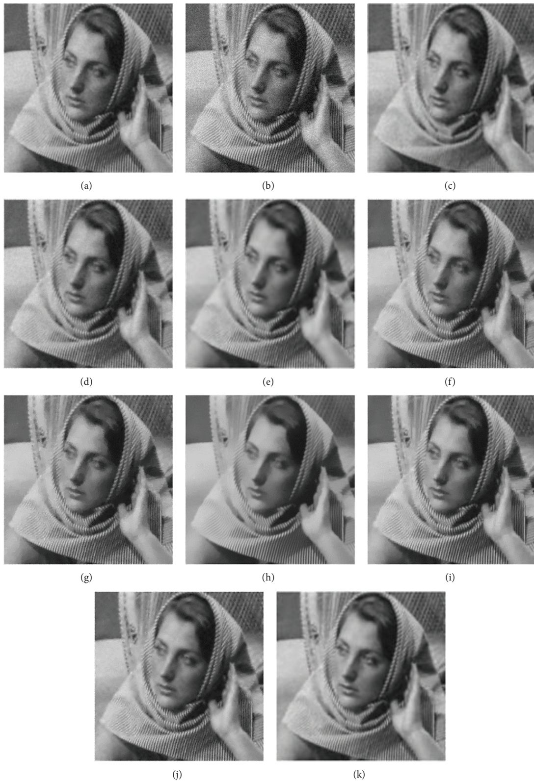
FIGURE 2: Comparison of the denoised results on “Barbara” image. (a) Original image. (b) Noisy image (additive Gaussian white noise, PSNR = 22.1 db). (c) PM model. (d) Fourth-order PDEs. (e) ZC model. (f) G-CDD. (g) BF. (h) NLMF. (i) BLS-GSM. (j) TGV. (k) Our proposed model.
