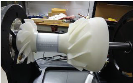
FIGURE 4: Low-speed axial-mixed compressor test rig without casing showing axial and mixed flow rotors.
