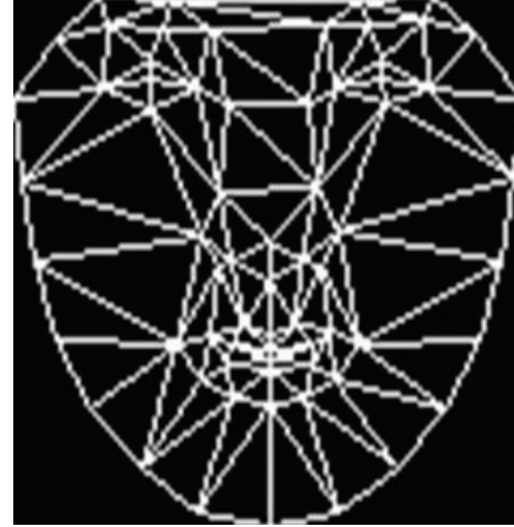
FIGURE 2: Result of the Delaunay triangulation.
