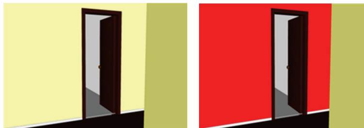
FIGURE 8: Chromatic alteration of the coating according to its state of deterioration.
