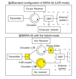
**Figure 1.** Simplified block diagrams of typical LDR (**a**) and hybrid (**b**) modes of MIRA-35. Components, added for the implementation of the hybrid mode from the LDR mode, are shown in yellow color. OMT is an orthomode transducer. See details in the text.
