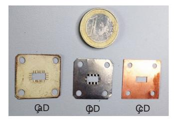
**Figure 2.** Throttle plates used for the phase adjustment. The thickness of the plates is 0.05 mm (**a**), 0.1 mm (**b**), and 0.28 mm (**c**). The introduced phase shift is  $1.8^{\circ}$  (**a**),  $3.4^{\circ}$  (**b**), and  $9.1^{\circ}$  (**c**).
