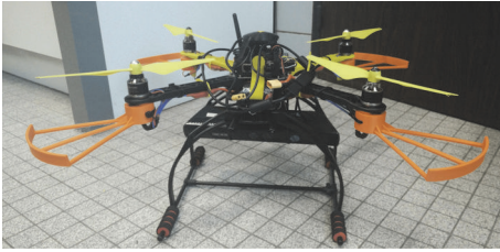
FIGURE 11: For our research, we mounted a Kinect camera to an Erl-Copter [10].
