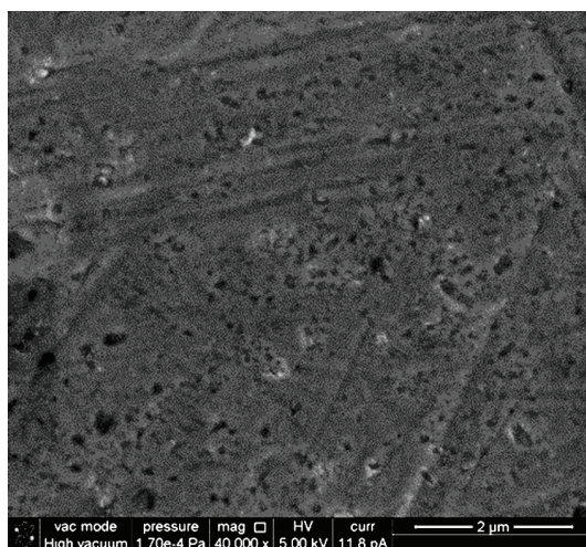
FIGURE 4: SEM micrograph for the nanolayer electrodeposited at 12 \text{mA}/\text{cm}^2 , in 1.1 M \text{H}_3\text{PO}_4 solution for 50 min.
