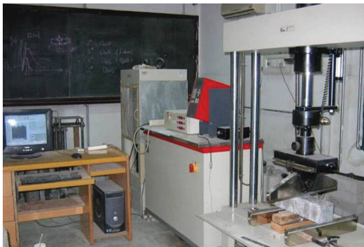
FIGURE 2: C120 high-performance concrete fracture parameter test.
