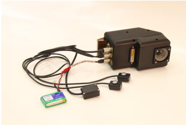
Figure 1. The FPI spectrometric imaging system including the camera, a 32 Gbyte compact flash memory card, two irradiance sensors, a GPS receiver and a LiPo battery
