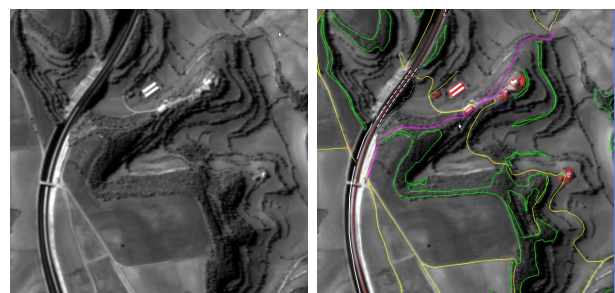
Figure 9. Example of data compiled using the Backward and Forward stereopair. Left: Original image. Right: Superimposed vector data including paved roads (red), unpaved roads (violet), paths (yellow), embankments (white), forests (green) and buildings (regular polygons in red).
