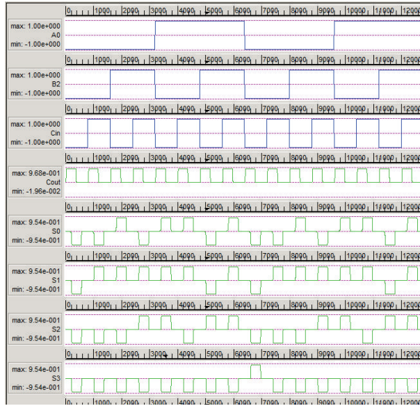
(b) Simulation result of 4-bit RCA
