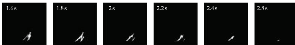
Figure 5: Photographs of flame quenching within the buffer area. It is different from the immediate effective concentration zone in Figure 4 as the flame cannot be suppressed directly, and the flame is smothered by the gradual increase of the aerosol concentration in the buffer area.
