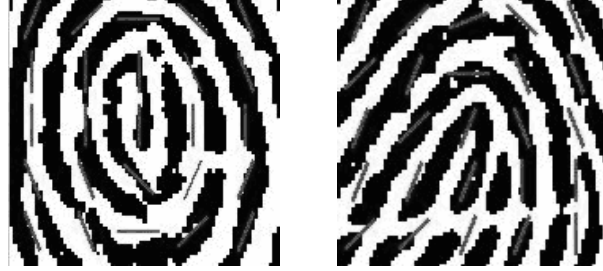
Fig. 9. The directional image of detected singularity regions overlapped with the fingerprint image.
